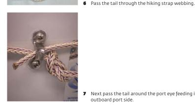
7 Next pass the tail around the port eye feeding it from the outboard port side.
