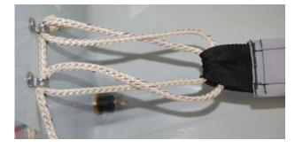
The rope tail is then passed through the starboard eye so that the end of the V12 can be pulled from the side of the boat.
