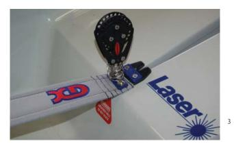
Fit new **XD hiking strap** and ratchet block using the spring and shackle provided.
